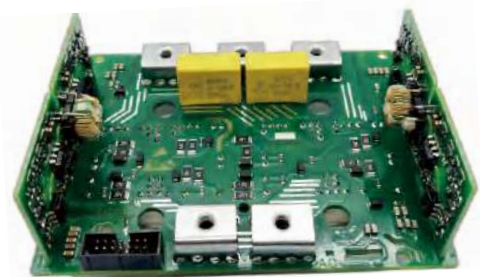
Two IGBTs in parallel installation unevenness <50um
